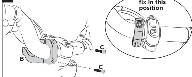
**Mount the bracelet (B) on the handlebar through the screws (C) without tightening.**
