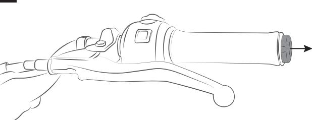
**Remove the originals counterweight and internal weight.**
