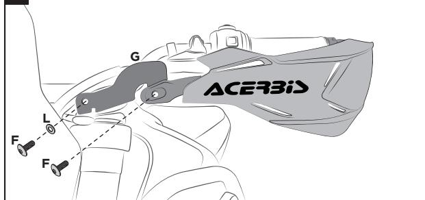
**Position the bracket (G) on the left side (on the right side use the bracket H) and fix through the screws (F) and the washer (L). Finally, tighten the bracelet.**
