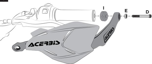
**Fix the handguard (A) to the handlebar using the counterweight (I), the bushing (E) and the screw (D) as shown in figure.**
